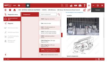
Wiring diagram configurations in the **EDC** engine control system of internal combustion forklifts of the **8FD Series** family, including images and component technical data.
