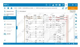
New wiring diagram configurations available for the **EMS10** engine control system.
