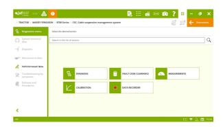
Autotronic 5 – TECU suspension control system in the front axle, activations, parameter configurations and calibration for 5700 S/SL Series, 6700 S Series, 7700 Series and 7700 S Series models.
