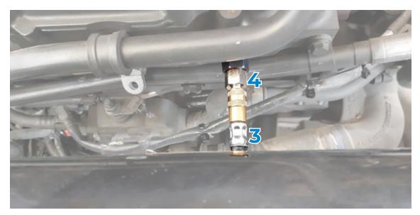
4 Adapter3 End of the test hose B
