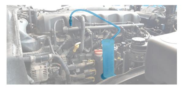
• Thread the blind cap **"2"** into the end of the pipe. Recommended tightening torque 30Nm.
