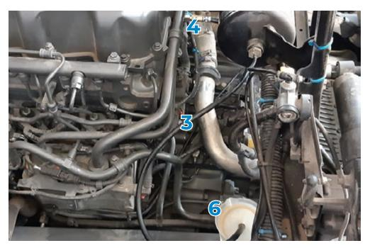
4 Adapter3 Test hose B6 Calibrated container
