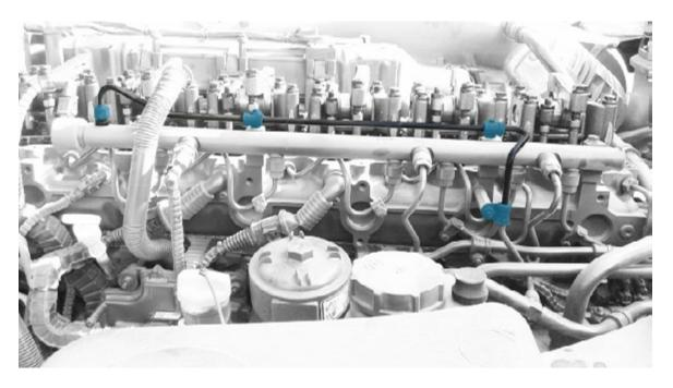
•Thread the test hose **"1"** into the connection of the rail fuel release pipe. Recommended tightening torque 30Nm. The other end of the hose should be inserted into a calibrated container for measuring the volume.
