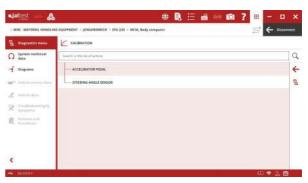
**MCM** central computer for **ETV 200** and **ETV 300** models, modification of the equipment parameters and the hydraulic system parameters, calibration of the accelerator pedal, etc.
