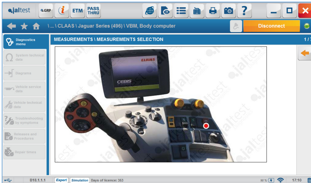
Image 16 Locations of the armrest switches in VBM system
