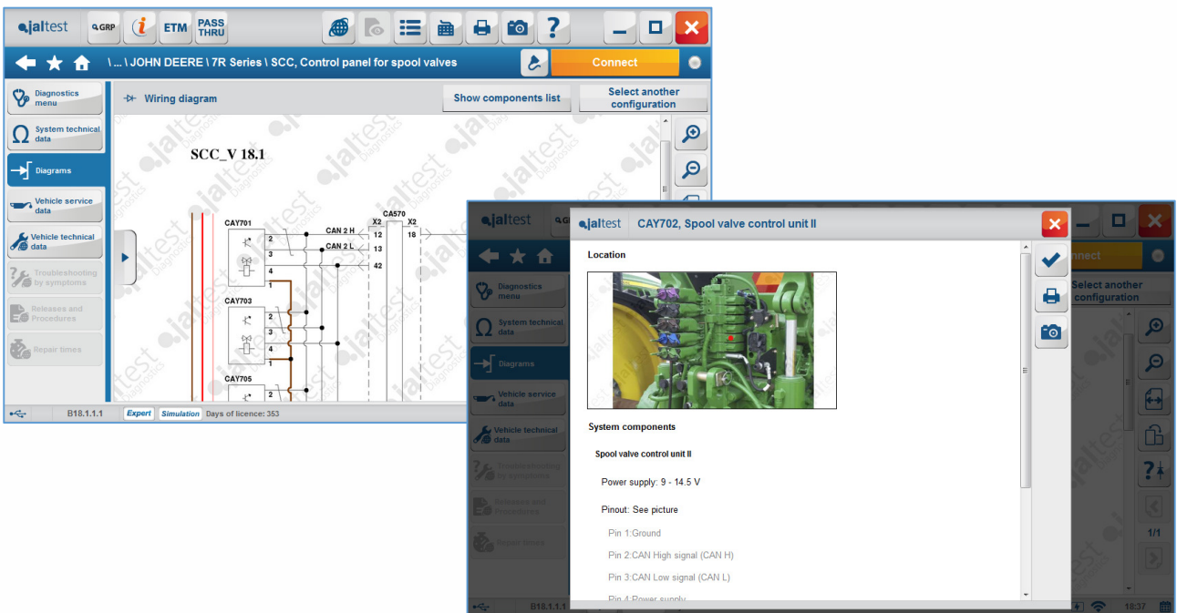
Image 32 Wiring diagrams and system technical data in SCC systems
