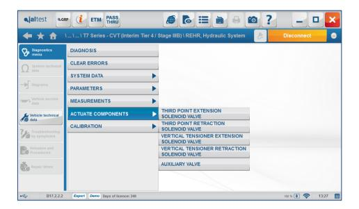
the user to check, exchange and replace the spool valves.
