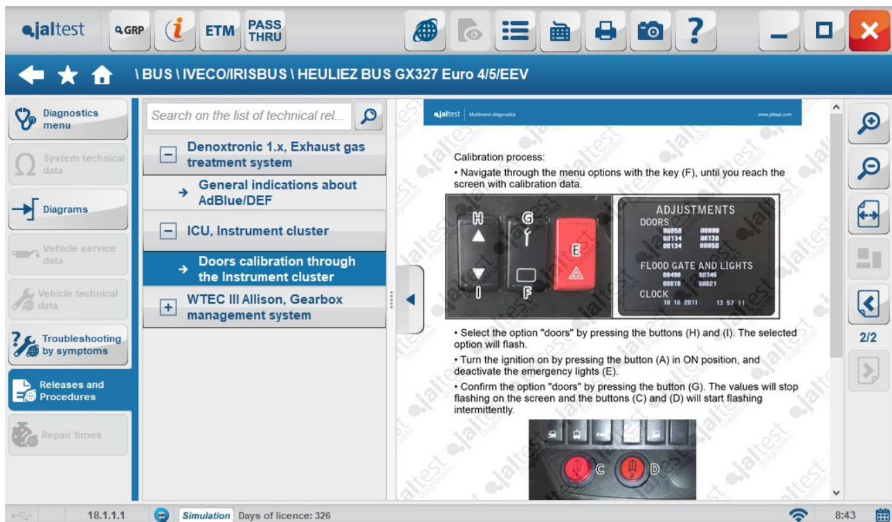
Image 19 Manual door calibration procedure in a Heuliez GX327 bus
