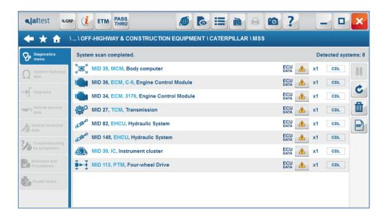
After this process of system detection and identification, the customer is provided with a list of the systems present in the machine. In addition, with this new function, the user of Jaltest can get a fast and intuitive overview of the possible faults and/or malfunctions present in the machine at a glance.
