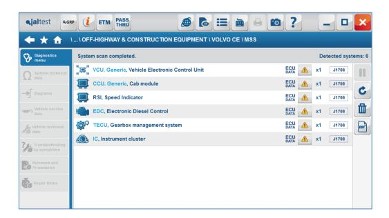
After this process of system detection and identification, the customer is provided with a list of the systems present in the machine. In addition, with this new function, the user of Jaltest can get a fast and intuitive overview of the possible faults and/or malfunctions present in the machine at a glance.
