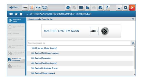
This new function allows the user to detect, connect and identify the different systems on the machine to be diagnosed, regardless of its model or application, thereby avoiding the process of identification of the machine and model.
