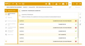
**VECU** Vehicle Electronic Control Unit in motor graders, transmission calibration.
