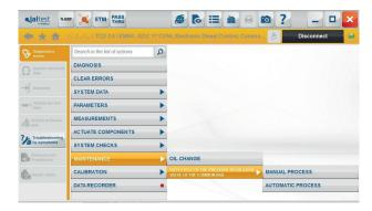
EMR4 engine management systems, service regeneration for CRT models in the EDC 17 CV52 system; injector coding, reset of the rail pressure regulation valve and much more in the EDC 17 CV54 system.
