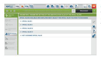
• New Sauer Danfos hydraulic system, which includes advanced functions such as the parameter setting of the spool valves identification code in Tier 3/Stage III & Interim Tier4/Stage IIIB models.
