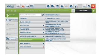
New functionalities of the Sisu Interim Tier 4/Stage IIIB & Final Tier 4/Stage IV engine management system, among which the following can be highlighted: the injector coding for 6-cylinder blocks and checks such as the cylinder cut-out and checks of the exhaust gases treatment system; the AdBlue/DEF dosing and the AdBlue/DEF pressure test.
