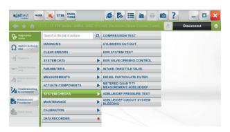
New functionalities of the Deutz EMR 4, EDC 17 CV52, engine management system, among which the AdBlue/DEF dosing and the AdBlue/DEF pressure test relating to the exhaust gases treatment system can be highlighted.
