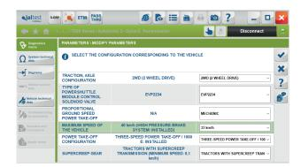
Parameter modification such as the maximum speed of the vehicle in the Autotronic 5-Dyna 6 transmission in X400, X600 & X700 Series models.
