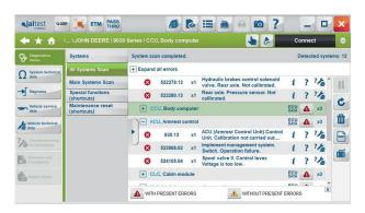
Software improvement based on the update of the System Scan results. If the status of the error memory of a system changes after accessing and repeating the reading process or clearing the errors, the System Scan results are updated. This way, for example, the report can be repeated with a more precise information about the vehicle status.
