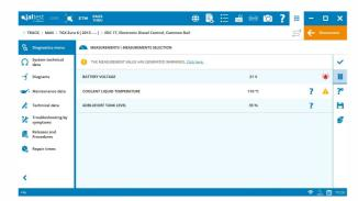
In addition to the different display methods available in Jaltest; the possibility to display measurements in graph format, define measurement triggers (also in measurement groups from this 21.1 version) and have measurement warnings during the display of them, now it is also possible to display a summary of slow-dynamic measurement warnings.
