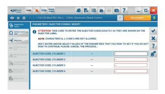
CDID3 engine management systems in Sprinter models and CR41 of Vito models with OM651 engine type, particulate filter reset and injector coding.
