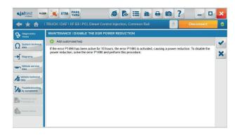
PCI KWP2000 (2013 – 2016) engine management system, MX engines, disabling of the power reduction caused by EGR error (it solves the P1495 error code).
