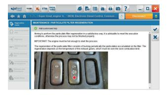
MCM engine management system for 6R10 engines, regeneration of the Diesel Particulate Filter (DPF).
